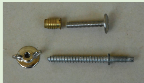
Figure 4-23. Many panels have permanent fastenings attached to the house. (i) After attaching the panel to the frame with two duplex nails (A), (ii) holes are drilled with the bit (B) into the panel and wood frame, (iii) then a spade wood boring bit (C) cuts wider holes into the panel and frame, (iv) and a lag screw anchor with female receptor (D) is screwed into the wood frame, (v) and the panel is attached with washer and wing nut (E).
